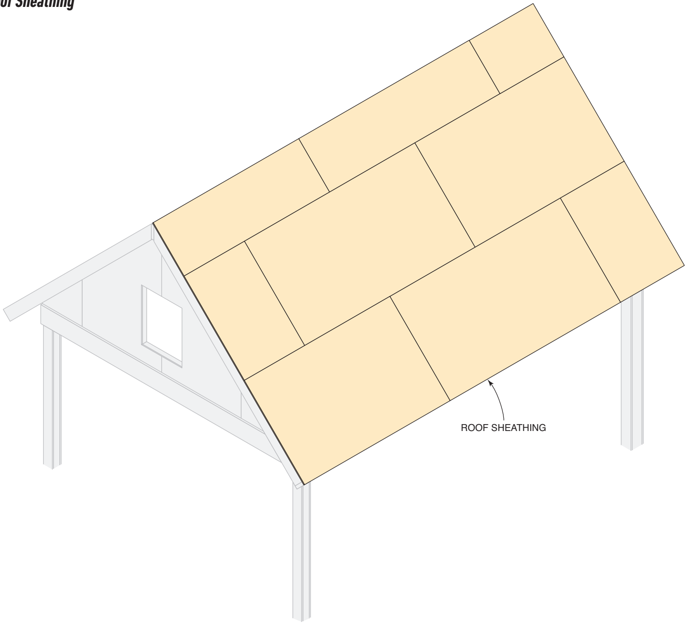
Figure N Roof Sheathing
